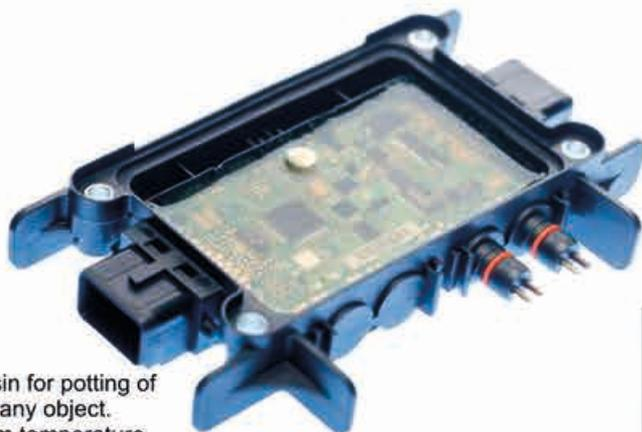
Transparent two-component epoxy resin for potting of sensors, processors, and back part of any object. Liquid, low viscosity, fast curing at room temperature with its suitable hardener. Good thermal conductivity, suitable for the encapsulation of electronic components, coils, transformers, easily workable after hardening.
