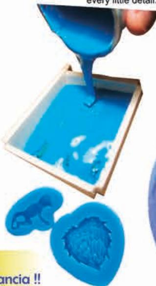
It is suitable to make monovalva moulds, of little, very detailed objects, even with strong undercuts, like statues, carvings, candles, etc.. With some devices you can also realize bivalve or cavity moulds, for reproducing more complex or larger objects. You can free download the brochure "Silicon rubber moulds construction" from our website Prochima.
