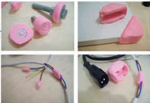
Two component, insulating paste rubber, moldable, flame retardant; Once mixed the 2 components in a 1:1 ratio (for not mote than 2 min.) and obtained a uniform compound, it rapidly cures at room temperature in less than 5 minutes.
